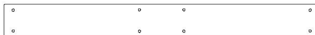
D01 | LISSE MURALE - W4L16426 (x1) | 1 3/8 po x 5 1/4 po x 50 3/8 po (36 x 134 x 1280)
