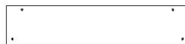
K05 | PLANCHE DE PLANCHER - W4L16449 (x1) | 5/8 po x 4 3/4 po x 20 7/8 po (16 x 120 x 529)
