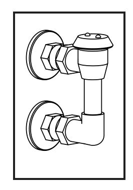
$\frac{3}{4}$ "[19mm]-3½"[89mm] 1/2" NPT FÉMALE OUTLET THREAD  $1\frac{1}{2}$ "[38mm] 37"+/- 1" -2X <sup>1</sup>/<sub>2</sub>"[13mm] [92mm +/- 3mm] 1/2" NPT FEMALE INLET THREAD SEE NOTE ALL DOTTED LINE PIPING IS SUPPLIED BY **OTHERS**  $2X \neq 2\frac{1}{2}$ "[ $\neq 64$ mm] SLIP FLANGE FINISHED WALL-
