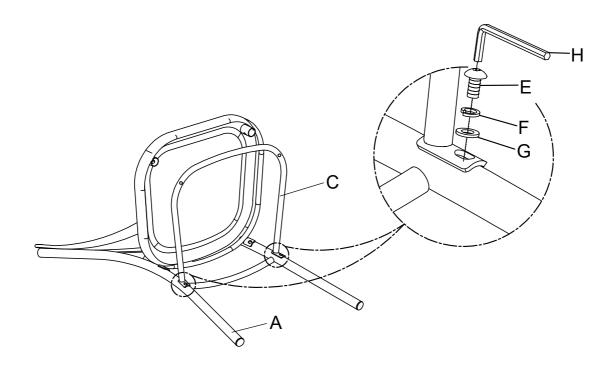
3 Attach Front Leg (D) to Seat (B), Stretcher (C) using Bolt (E), Lock Washer (F), Flat Washer (G) by Allen Key (H).
