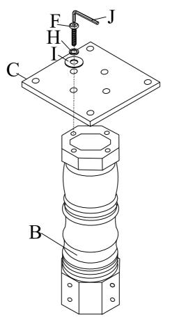
2 Attach the Mounting Plate (C) to Table Top (A) with Flat Washer (I), Lock Washer (H), Bolt (E) and fully tighten with Allen Key (J). Do not over tighten.
