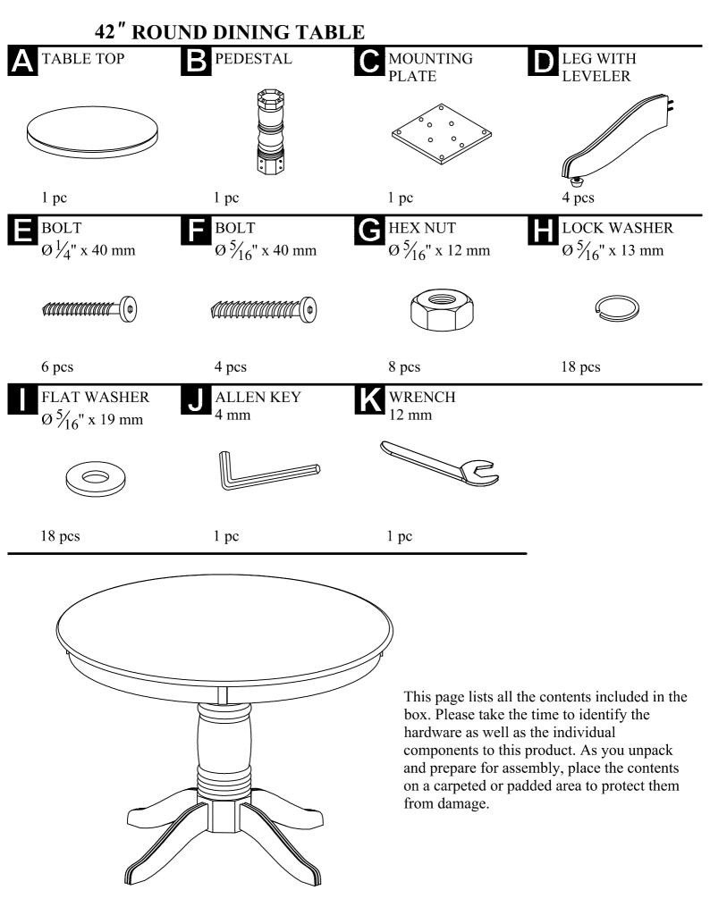
Attach the Mounting Plate (C) to Pedestal (B) with Flat Washer (I), Lock Washer (H), Bolt (F) and fully tighten with Allen Key (J). Do not over tighten.
