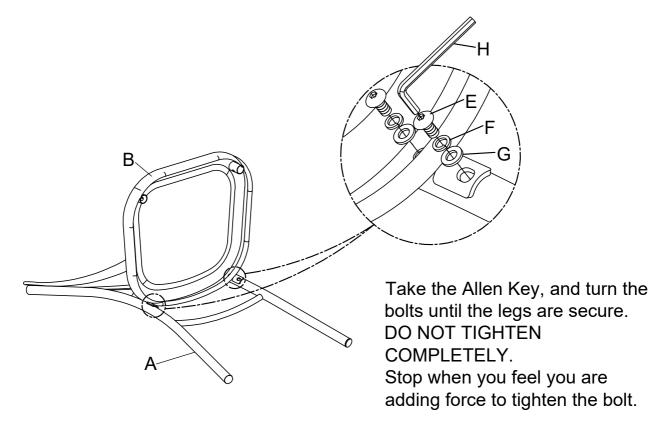
2 Attach Stretcher (C) to the Chair Back (A) using Bolt (E), Lock Washer (F) and Flat Washer (G) by Allen Key (H).
