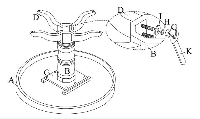
4 Turn the Table to upright position, place it on flat surface and adjust the Leveler so that Table is level and does not wobble. Assembly product is now completed.
