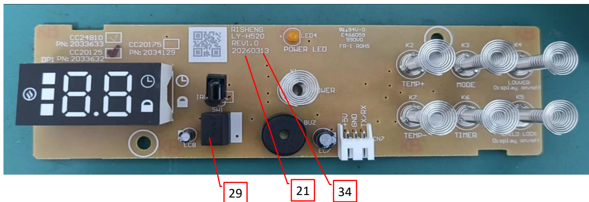
Photo 28 - Risheng Display PCB for model CC20125
