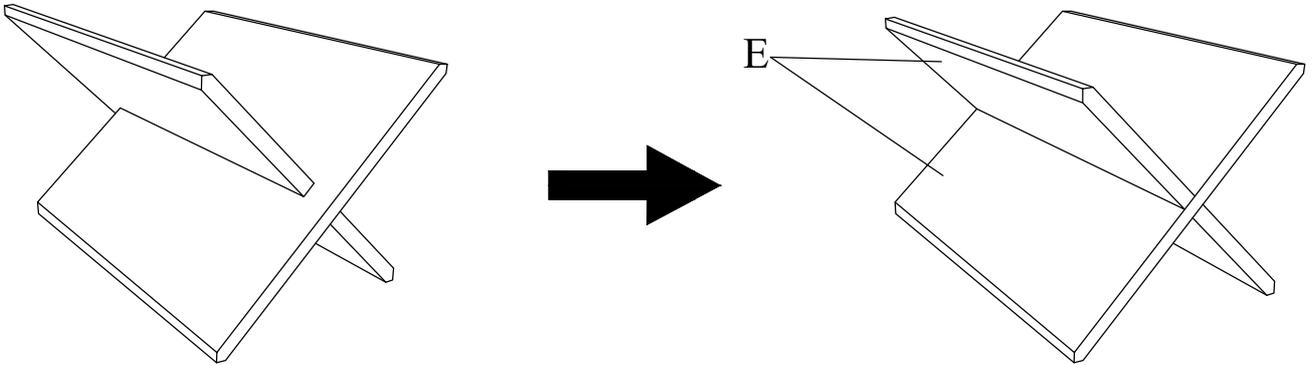
**3** Use PVC Dowel (K) as a guide, align and attach Divider (C) to Upper & Lower Shelf (B & D), then tighten Mini Fix Housing (M) with Allen Wrench (O).
