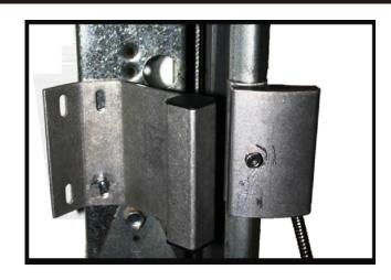
Model DC-4811 provides an effective and convenient means to secure panel type roll up doors which incorporate a roller track transport mechanism. The inclusion of an adjustable L-bracket allows fitting to roller tracks up to 3in wide. For the highest level of security, mount the switch below any other devices installed on the track while still high enough to keep the cabling off the floor surface.
