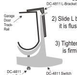
2) Slide L bracket into the switch so it is flush to flat side of the rail.
