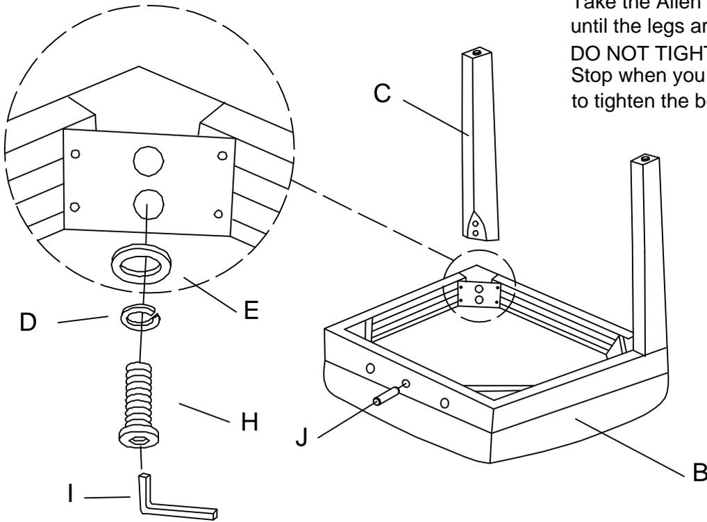
Take the Allen Wrench, and turn the bolts until the legs are secure.
