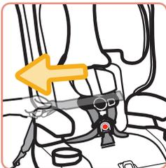
For the **LATCH belt or Lap Only Vehicle Belt**: it may be easier to tighten if you route the free end of the belt back into the **Forward-Facing Belt Path**, reach into the **Forward-Facing Belt Path**, and pull the free end of the belt towards you.
