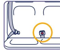
When using the belt-positioning clip, it **must be** installed on the side of the booster seat that is closest to the vehicle seat buckle.
