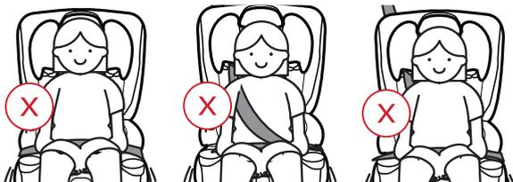
Use **ONLY** the vehicle's lap and shoulder belt system when restraining the child in this booster seat.
