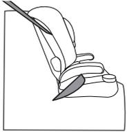
Keep the booster seat securely belted through the belt-positioning guide even when unoccupied.
