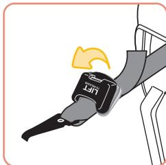
Lift Tether Adjuster to Loosen Tether Strap
