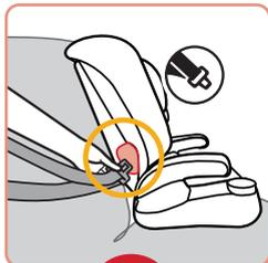
Locate **Forward-Facing Belt Path** & Route Vehicle Belt or Lower Anchor Belt Through It
