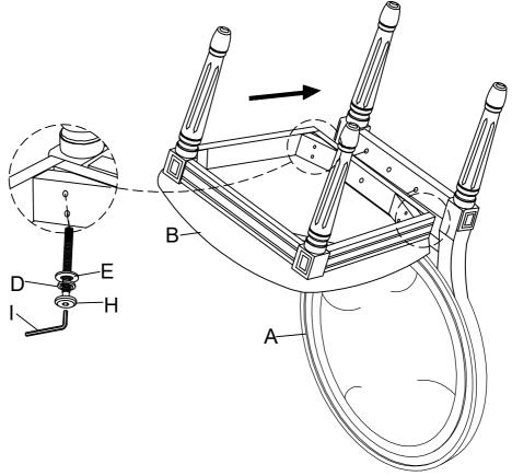
Finally, assemble the last Bolt (F) to Seat (B) and Chair Back (A) with Lock Washer (D) & Flat Washer (E) by Allen Key (I).
