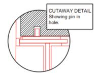
TO ACCOMMODATE THE HINGE PINS ON THE HINGE SIDE OF THE PANEL Drill a hole at least 5/16" in diameter and 1" deep into the top and bottom of the frame in the location shown.
