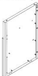
S7 FRIDGE CABINET SIDE PANEL ASSEMBLY L - A4M03597 (x1) 33 7/16"x23 3/8"x2 1/16" (53x594x849.7)
