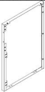
S3 SINK CABINET SIDE PANEL ASSEMBLY L - A4M04538 (x1) 33 3/8"x23 3/8"x2" (50x594x848.2)
