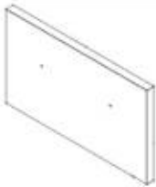
D3 CABINET DRAWER PANEL ASSEMBLY - A4M03569 (x1) 17 3/4"x10 1/4"x15/16" (24x260x451)
