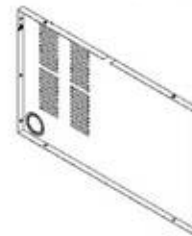
G10 CABINET BACK PANEL ASSEMBLY - A4M03055 (x1) 1 3/16"x22 7/8"x38 3/16" (30x581x970)
