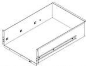
D4 CABINET DRAWER BODY ASSEMBLY - A4M03571 (x1) 22 1/4"x16 1/16"x6 7/16" (164.2x408.4x565.4)
