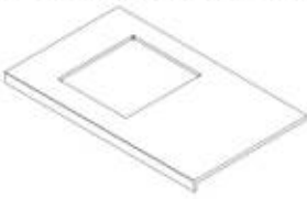
M2 SINK CABINET MARBLE - A4M03568 (x1) 41 1/2"x24 15/16"x1 15/16" (49x633x1054)
