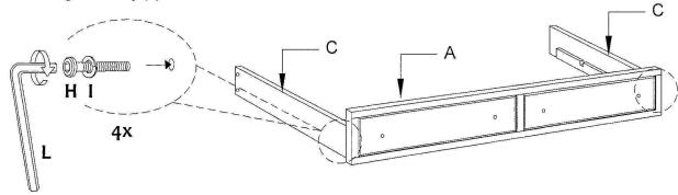
Attached Side Frame (C) to Back Frame (B) by inserting JCBC Bolt (H) with Spring Washer (I) into provided holes using Allen Key (L).
