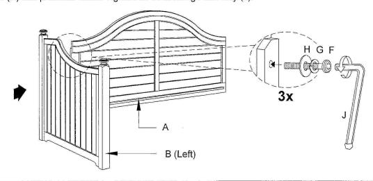
Attached Side Frame (C) (Right) to Back Panel (A) by inserting JCBC Bolt (F) with Spring Washer (G) and Flat Washer (H) into provided holes. Do not tighten the bolts. Insert Front Rail (D) to Side Frame (B) (Left). Repeat the same process to Side Frame (C) (Right). Then tighten all the bolts using Allen Key (J).
