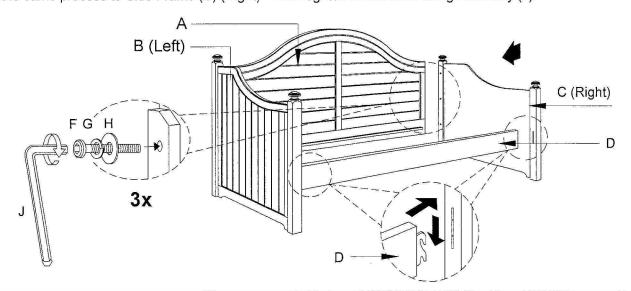
Place Slats (E) to the Back Panel (A) and Front Rail (D). Secure the Slats (E) with Spring Washer (G) and JCBC Bolt (F) and tighten using Allen Key (J) & CSK Screw (I) following the diagram below.
