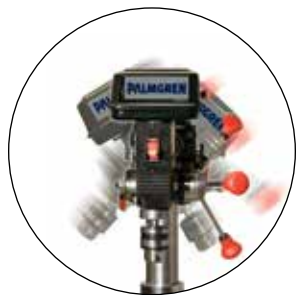
The head tilts 90° left and 45° right.
