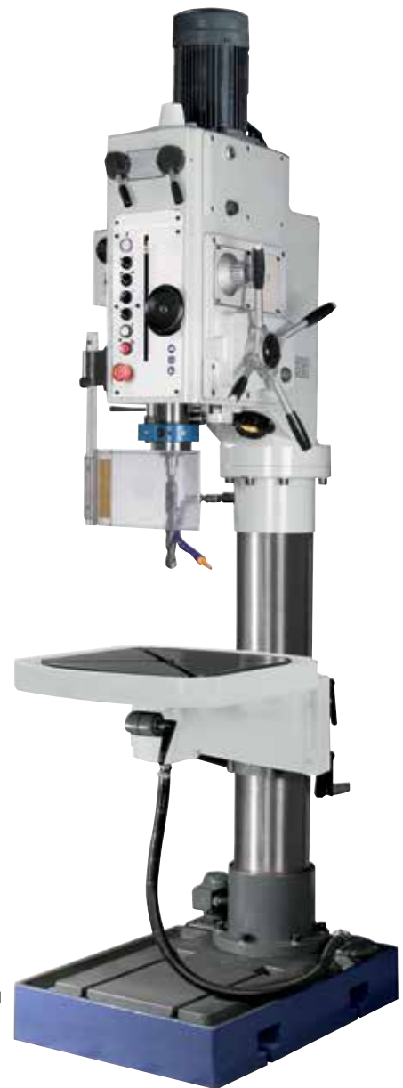
9 selectable speeds via gear shifting lever at the front of the drill head combined with a two-stage motor provides 18 spindle speeds
