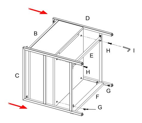
Attach Top Panel (A) to the Side Frame - LSF (C) and Side Frame - RSF (D) by using Bolt (G) and Allen Wrench (I) as shown.
