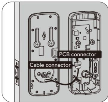
8. Install interior assembly on inside mounting plate.
