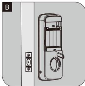
Using a pointed object, press and hold the reset button for over 5 seconds.
