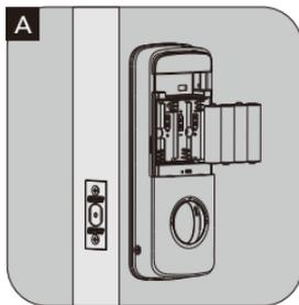
Keep your lock in "unlock" status, insert 4x AA batteries in battery pack.
