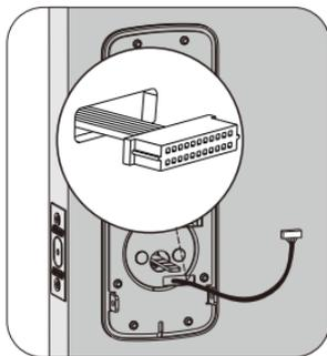
6. Secure both assemblies using the screws provided. Make sure the exterior assembly is vertically aligned. If you added the cross bolt, securely tighten the post to the exterior Ease unit with the additional screw provided.
