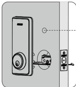
This hole is for the optional cross bolt provided for stabilising your lock. If you drilled a hole, securely tighten the post before mounting on the door.
