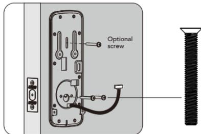
7. Attach cable assembly to the interior assembly PCB by lining up notches on top of cable connector to slots on PCB connector. Press connector in firmly until completely connected.
