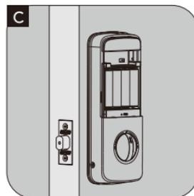
If reset is successful, the latch bolt will extend on its own to learn the orientation of the door.
