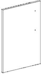
D1 CABINET DOOR PANEL ASSEMBLY L - A4M03546 (x1) 28 7/16"x19 5/8"x15/16" (24x498x722.5)
