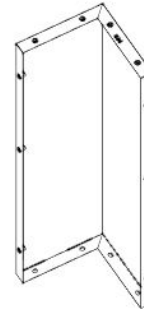
S34 CABINET CORNER PANEL ASSEMBLY - A4M04850 (x1) 33 3/8"x8 11/16"x8 11/16" (220x220x848)
