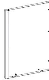
S21 CABINET SIDE PANEL ASSEMBLY L - A4M04670 (x1) 33 7/16"x23 3/8"x1 3/8" (35.00x594x849.7)
