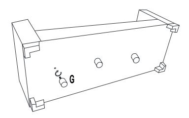
Hook on the Back Frame (B) to Left Panel (C) & Right Panel (D) properly.
