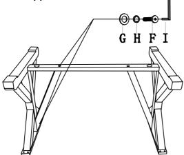
Attache Leg(B) to Top(A) by using screw(E), flat washer(G), spring washer(H) and allen washer (I) as shown.
