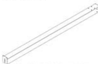
P02 FRONT POST - A4M02977 (x1) 4 3/4"x6 1/8"x96 5/8" (120x155x2455)
