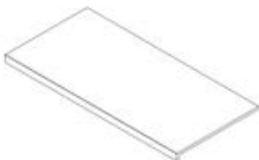
M1 CORNER CABINET MARBLE - A4M03035 (x2) 1 15/16"x24 13/16"x51 7/8" (50x630x1317)
