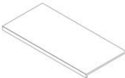
M1 CORNER CABINET MARBLE - A4M03035 (x1) 1 15/16"x24 13/16"x51 7/8" (50x630x1317)
