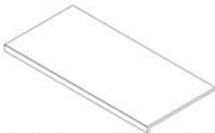
M1 CORNER CABINET MARBLE - A4M03035 (x1) 1 15/16"x24 13/16"x51 7/8" (50x630x1317)
