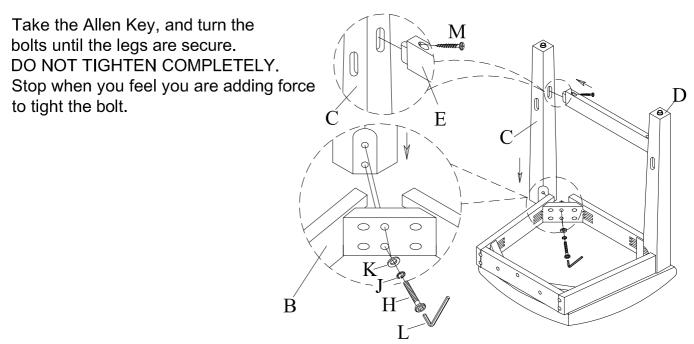
Insert dowels to the back rail of seat (B) then attach the seat frame to the chair back(A) using flat washer (K), lock washer (J), bolt (G), (I) by allen key (L). Do not too tight.
