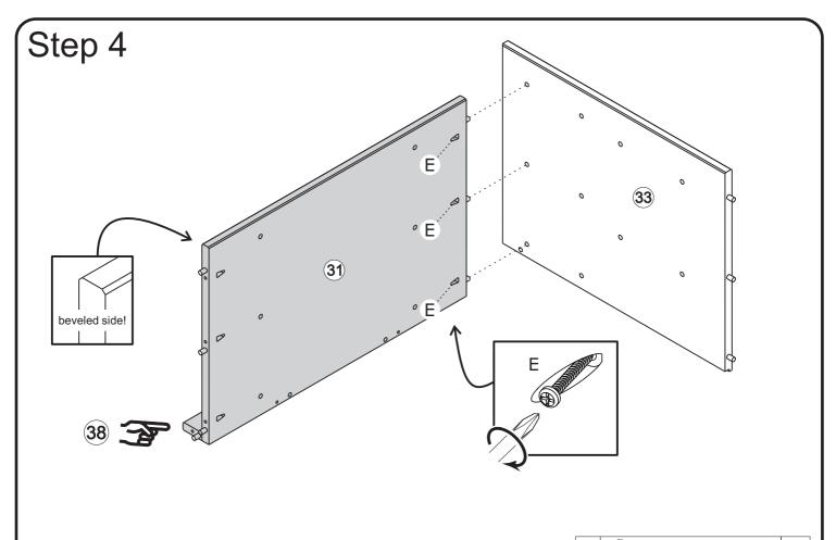
Secure part (31) and (38) to part (33), attach part (31) to part (33) with screw (E) and screwdriver (not included).
