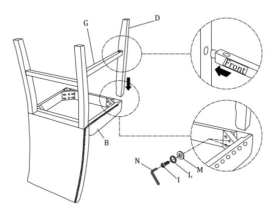
3 Attach the Front Left Leg (C), Left Stretcher (F) and Front Stretcher (E) to the Chair Seat (B) using Screw (K) with a Phillips head screwdriver (not provided). Attach the Front Left Leg (C) to the Chair Seat (B) using Allen Bolt (I), Spring Washer (L) and Flat Washer (M) with Allen Key (N).
