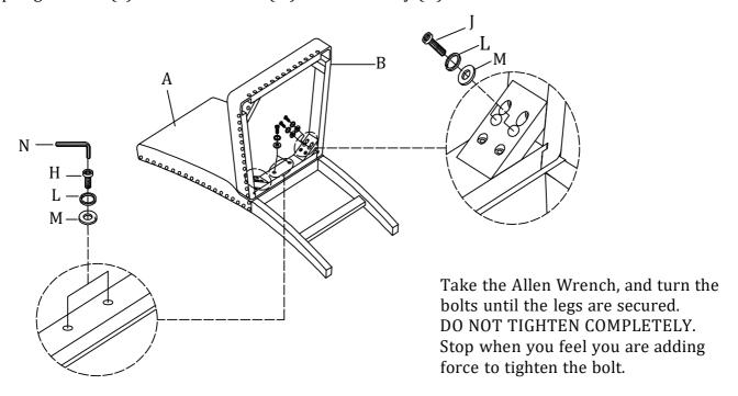
2 Attach the Front Right Leg (D) and Right Stretcher (G) to Chair Seat (B) using Allen Bolt (I), Spring Washer (L) and Flat Washer (M) with Allen Key (N).
