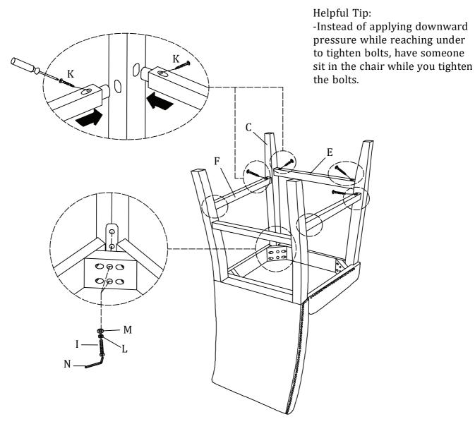
Stand chair up on an even surface and check that it is balanced. If there is a slight wobble, apply downward pressure in the corner where a leg is uneven. Keeping pressure in that corner, tighten all bolts. If balanced, apply downward pressure evenly in the center and tighten all bolts. Do not over tighten beyond hole depth.
