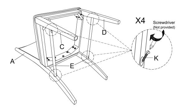
Stand the chair on an even surface and check for balance. If the chair wobbles slightly, apply downward pressure on the uneven leg and tighten the bolts to correct the imbalance. Once the chair is balanced, apply downward pressure evenly in the center of the chair and tighten all bolts, being careful not to over-tighten beyond the hole depth.
