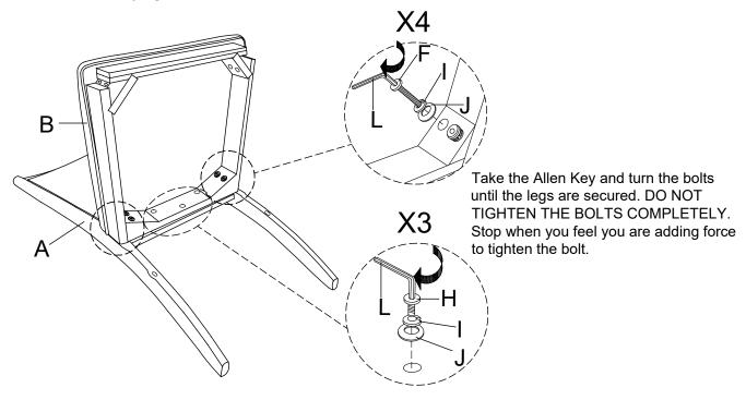
Attach the Left Front Leg (C) and the Right Front Leg (D) to the Cushion Seat (B) using JCBC Bolt (G), Lock Washer (I) and Flat Washer (J) with the Allen Key (L).
