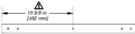
J3 | MONTANT MURAL - W4L12396 (x1) | 1 po x 2 3/8 po x 36 1/2 po (24 x 60 x 927)
