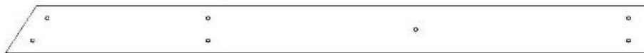
G1 | PLANCHE DE SOL - W4L12290 (x1) | 1 po x 5 1/4 po x 70 3/4 po (24 x 134 x 1 798)
