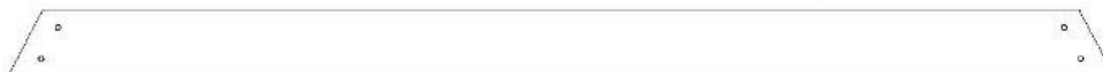
G16 | PLANCHE DE SOL - W4L12442 (x1) | 1 po x 5 1/4 po x 86 3/4 po (24 x 134 x 2 202)
