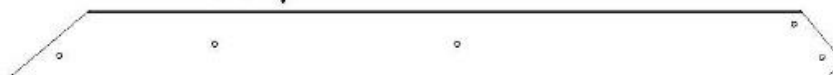
G13 | SUPPORT TRANSVERSAL - W4L12314 (x1) | 1 po x 5 1/4 po x 65 1/4 po (24 x 134 x 1 658)
