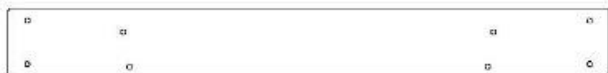
G6 | RAIL DE PLATEFORME - W4L12295 (x1) | 1 po x 5 1/4 po x 47 po (24 x 134 x 1 194)
