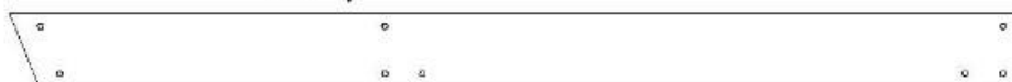
G4 | PLANCHE DE SOL - W4L12293 (x1) | 1 po x 5 1/4 po x 72 1/4 po (24 x 134 x 1 835)
