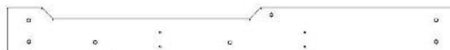
G5 | RAIL DE PLATEFORME - W4L12294 (x1) | 1 po x 5 1/4 po x 51 po (24 x 134 x 1 296)
