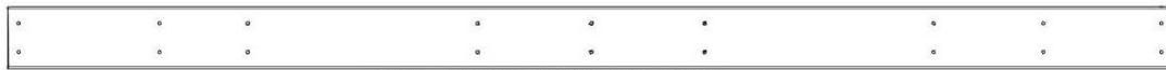
OG09 SOLIVE DE PLANCHER - W4L22485 (x2) 1 3/16 x 3 3/8 po x 63 1/16 po (30 x 86 x 1602)
