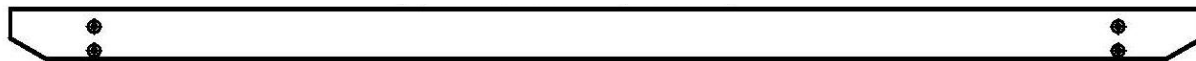
E01 PLANCHE DE GARNITURE - W4L22459 (x2) 1 7/16 po x 3 3/8 po x 78 1/8 po (36 x 86 x 1984)
