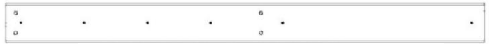
OR01 MONTANT VERTICAL - W4L22406 (x2) 1 3/16 po x 2 3/8 po x 28 3/4 po (30 x 60 x 730)
