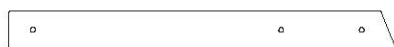
F5 | PLANCHE DE SOL - W4L12488 (x1) | 1-3/8 po x 2-3/8 po x 24-1/4 po (36 x 60 x 617)
