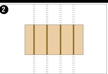
Once the installation location and studs have been identified, enough drywall must be cut away to expose the underlying studs with enough space for reframing to take place.
