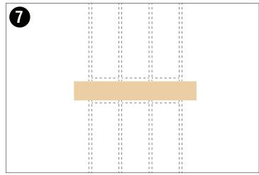
After the wall has been braced, sheetrock must be cut to size to cover the reframed area. The sheetrock must also have a section cut to accomidate the QX frame and SoundBar. After the drywall has been secured to the wall, mudding can be performed to cover any installation seams and retexturing can be done to blend it to the installation area.
