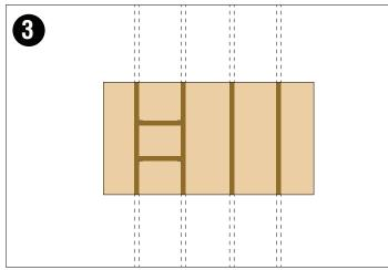
Once the drywall section has been removed, the the studs are now free to be braced and  $\operatorname{cut}\nolimits$
