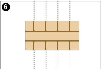
Continue the reframing process until the required length to accommodate the QX SoundBar has been reached.
