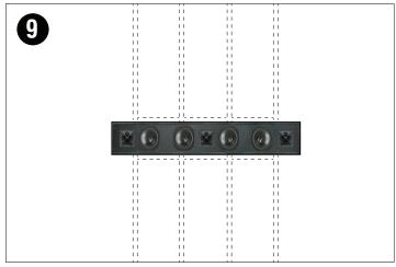
Once the frame is securely mounted to the dry wall, the SoundBar can be wired, inserted and secured to the frame.
