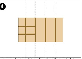
We recommend bracing each stud on both sides, with your method of choice, before performing cuts on the vertical wall studs.
