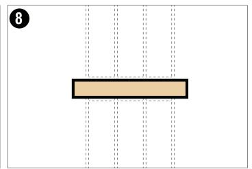
After the mudding process is complete and dry, the QX SoundBar's frame can be installed and clamped onto the dry wall.
