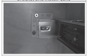
Once door is installed and aligned, cycle the unit a couple of times making sure the soft-close is working correctly. Then open the unit all the way and install into the center of each of the self-adjusting rear brackets one (1)  $\#8 \times 1/2$ " Pan Head Phillips Wood Screw to hold the bracket in place. Install trash cans.
