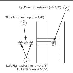
To adjust door up or down loosen door mounting screws (A). To adjust left or right, loosen both set screws (B) adjust and retighten. To adjust tilt, loosen both set screws (B) and then turn tilt screw (C) clockwise to desired distance and then retighten set screws.
