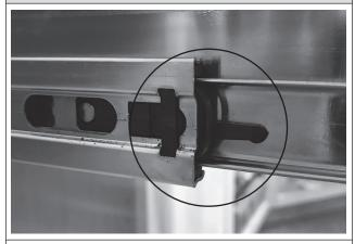
Separate the slides using the black separation arms shown above. Install cabinet member of the slide at your desired mounting location with one (1) #8 x 1/2" Pan Head Phillips Wood Screws provided.
