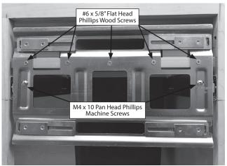
Placing the Wood Top Assembly on a flat surface, place the Door Mounting Metal Frame on the Wood Top as shown above and align with the pre-drilled holes. Secure in each location shown with #6 x 5/8" Flat Head Phillips Wood Screws provided. Then install the two (2) M4 x 10 Pan Head Phillips Machine Screws into the front of the slides brackets as shown.
