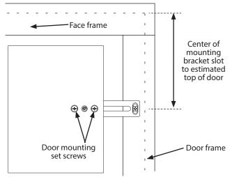
Loosen the door mounting set screws and slide bracket out to desired position to attach to the door rail. Measure from the center of the slot on the door mounting bracket to the estimated top of door. Mark door with measurement for both top brackets. Install door with the four (4) #8 x 5/8 Flat Head Phillips Wood Screws provided. (NOTE: DETERMINE CORRECT SCREW LENGTH TO DOOR PANEL THICKNESS.) Double sided tape included with hardware to assist with door installation.
