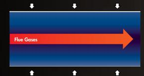
Vortex™ turbulator inside the heat exchanger increases efficiency by disrupting the natural airflow which extracts the maximum heat from the flue gases.
