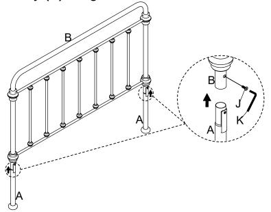
Insert the Front Rail Section (D) to the Rear Rail Section (E), and then insert the Bolt (J), turn the L-Allen Key (K) to tighten them.
