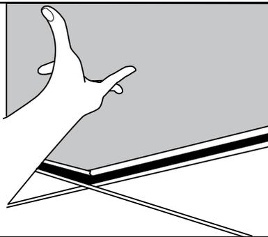
5 Remove access plate from junction-box (do not discard) by removing screws.
