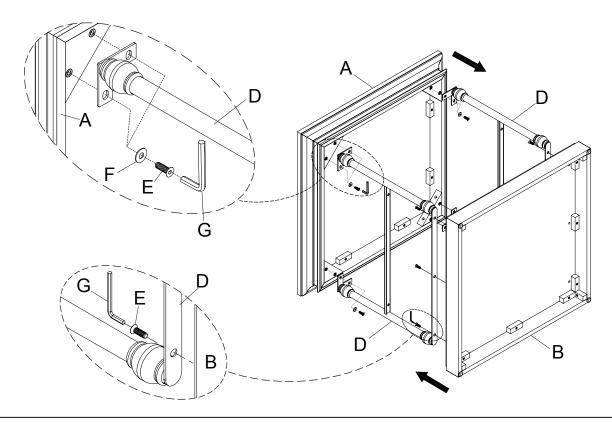
Assembly the Shelf (C) onto the Side Frame (D) and using the Bolt (E) by Allen Wrench (G).
