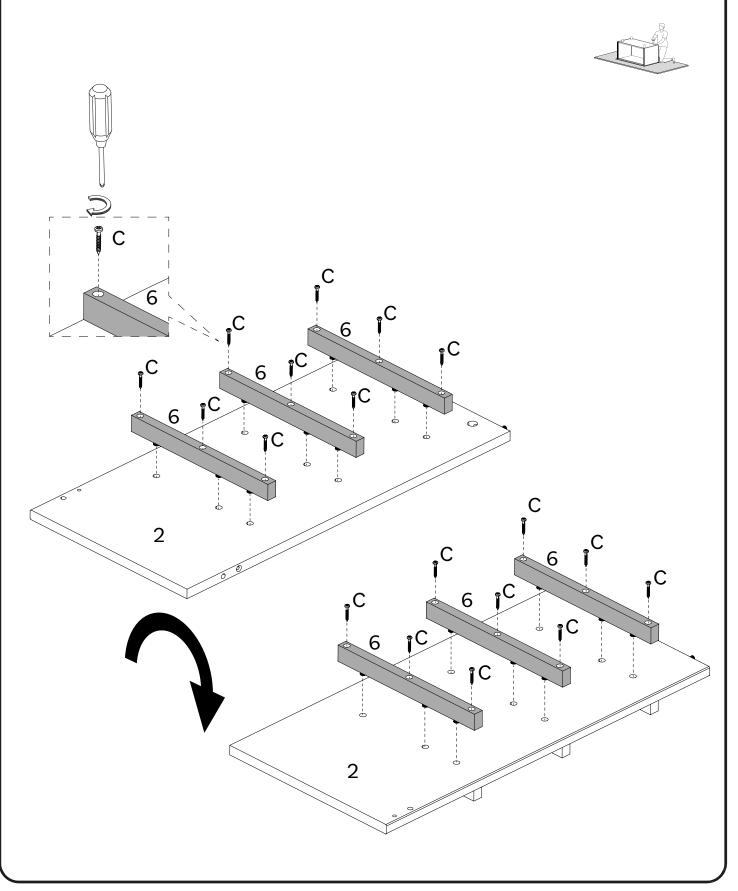
Attach Wood Sliders (6) to the Left Panel (4) and Right Panel (8) using (C) Screws.
