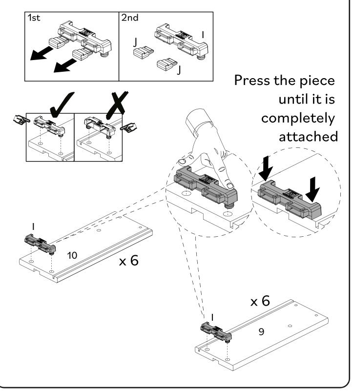
You're almost done! Slide the Dovetail (I) on the Right Drawer Panel (9) and the Left Drawer Panel (10) into the grooves on the Drawer Front (11). Repeat this for all drawers.
