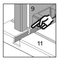
Align the grooves on the Drawer Sides and Drawer Front to receive the Drawer Bottom
