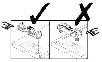
TIP: We've made it easy with a illustration on the drawer fronts to show the correct direction for the Dovetail.
