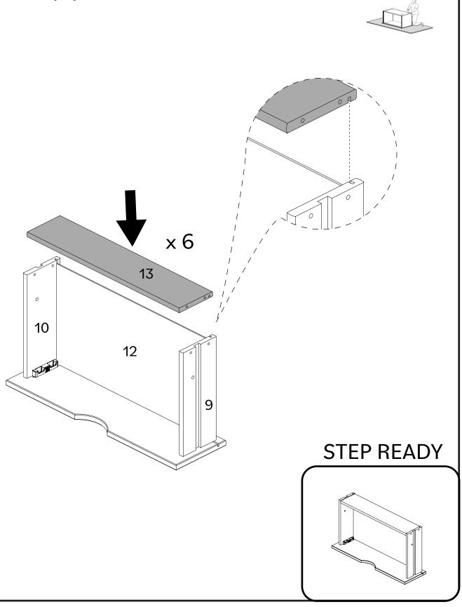
Secure the Drawer Backs (13) by inserting the Plastic screws (K). Use a hammer if necessary. Slide the finished drawers into the dresser.
