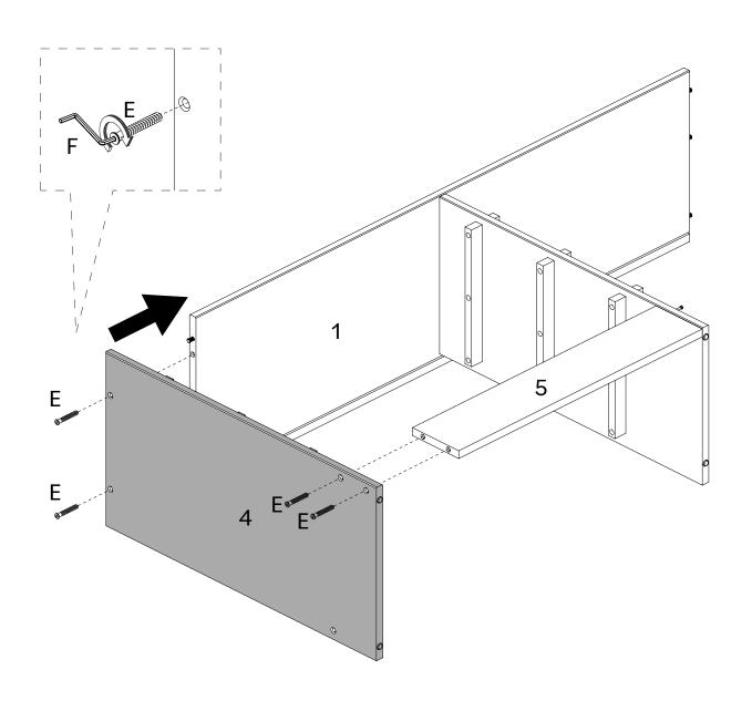
Make sure your unit is right-side up (Top Panel (1) on top). Attach the Back Rail (3) to the Left Panel (4) and Middle Panel (2). Secure with (E) Bolts and the Hex Key (F)!
