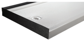
Factory-installed tile flange is 1/16" thick. Account for this thickness when planning final opening size.
