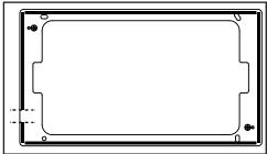
Cut a piece of the adhesive strip where the lightning cable will route behind Surface Mount.
