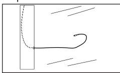
Drill a 3/8" small hole and route the lightning cable down the aluminum channel and out the hole. Make sure there is enough length.
