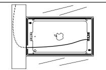
Connect the iPad and place it in the bezel. (See Surface Mount Instructions) Attach the bezel to the bracket. Adhere the Surface Mount to the glass close to the channel.
