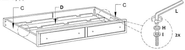
Attached Castor Wheel (J) to two Center Rail Support (E) (Short) with CSK Screw provided. Put the Center Rail Support (E) (Short) following the diagram below and secure it with JCBC Bolt (H) & Spring Washer (I) using Allen Kov (L)
