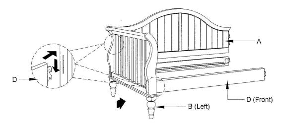
Attached Side Frame (C) (Right) to Back Panel (A) and Rail (D) (Front & Back).
