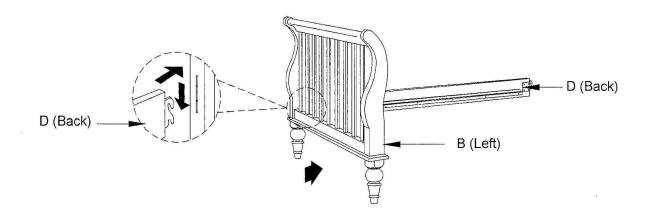
Attached Side Frame (B) (Left) to Back Panel (A) and Rail (D) (Front).
