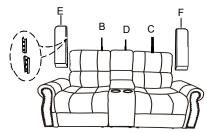
STEP 2:Install the LSF backrest (B), Console back (D), and RSF backrest (C) by align and insert the metal bracket to the metal brackets of the seat (A).Connect the wire between the backrest (B) and backrest (C) with the wires on seat (A).Please make sure the brackets are inserted all the way and secured into position
