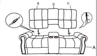
STEP 4: Connect the power and open/close the footrest by pressing the button.
