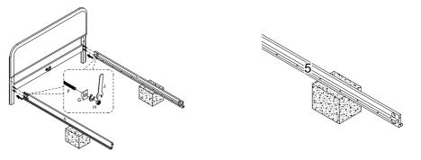
Repeat that same process to finish off the frame. Place the bolts in the Curved Corner Pieces (7) into the Side Rails (5) and secure with the Half-moon washers (G) and Nuts (H).
