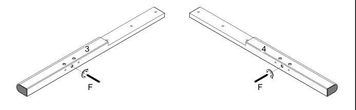
Turn over the Headboard Posts (3 & 4) and insert the bolts into to the Headboard Support Rail (2). Secure with a Halfmoon washer (G) and Nut (H) then tighten with the Wrench (J).
