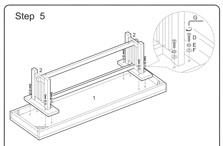
Attach leg pieces (2) to bench top (1) using bolts (D), spring washers (E) and washers (F). Tighten all bolts (D) with wrench (G).
