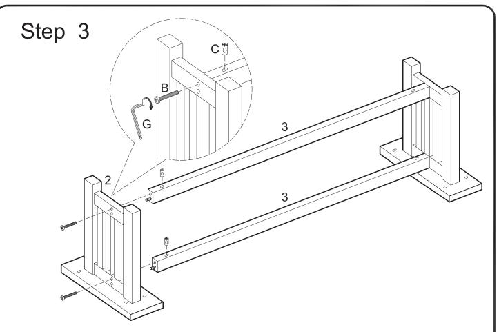
Insert nuts (C) into opposite ends or crossbars (3). Attach crossbars (3) to second leg piece (2) using bolts (B). Tighten bolts (B) with wrench (G). Bolts (B) will screw directly into nuts (C).
