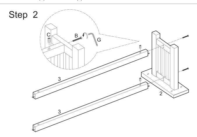
Insert nuts (C) into crossbars (3). Attach crossbars (3) to leg piece (2) using bolts (B). Tighten bolts (B) with wrench (G). Bolts (B) will screw directly into nuts (C).
