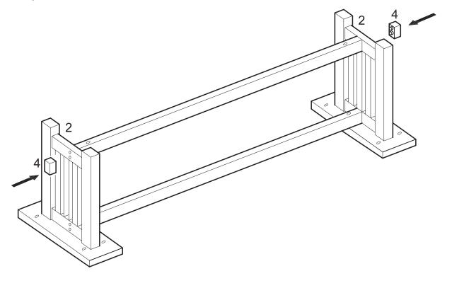
Insert end caps (4) into leg pieces (2) using pre-inserted dowels as guides
