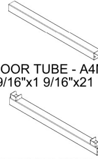
F09 BOTTOM FLOOR TUBE - A4M02210 (x1) 1 9/16"x2 3/8"x21 7/8" (40x60x555)
