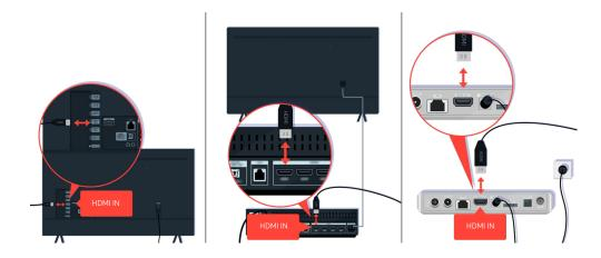
Check the antenna and HDMI cable connections.
