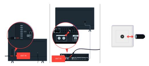
Check the antenna and input cable connections.
