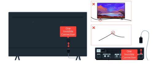
If the problem persists, and if your TV uses the One Invisible Connection, disconnect and reconnect the One Invisible Connection to the TV and the One Connect (OC) Box. Ensure that the One Invisible Connection is not pinched or bent sharply.
