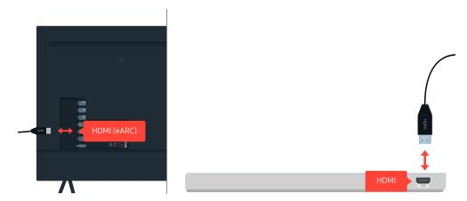
If no sound comes out of your Sound Bar, and if it is connected to the TV with an HDMI cable, check the HDMI (eARC) connector on the back of the TV.
