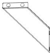
C01 CORBEL ASSEMBLY - A4M05701 (x5) 12 1/8"x3 3/4"x2" (50x95x309)
