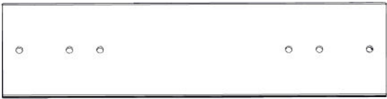
W14 ROCK WALL BOARD - A5C00009 (x2) 29 5/16"x5 1/2"x7/8" (23x140x744)
