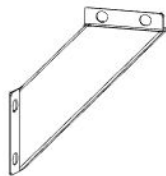
C02 CORBEL ASSEMBLY - A4M05702 (x5) 12 1/4"x3 3/4"x1 15/16" (50x96x309)
