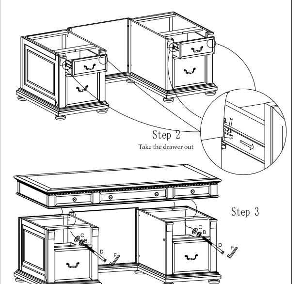
Step 2: Remove the upper drawers in both pedestals - Open drawer fully to expose the release levers in the center of the drawer slide. Push the lever on the left side up, and the lever on the lever on the right side down to release drawer. With levers pushed gently tug the drawer out of the desk
