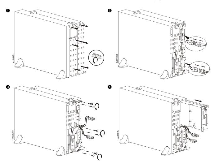
Disconnect and remove the battery module from the UPS. See "Tower to rack-mount conversion" on page 3.
