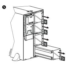
Oisconnect and remove the battery module from the UPS. See "Tower to rack-mount conversion" on page 14.
