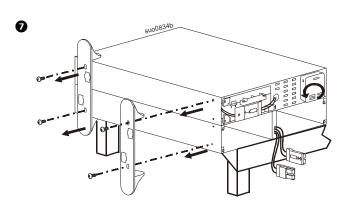
Install the SRT1000/SRT1500/SRT2200/SRT3000 UPS with one external battery pack in a rack
