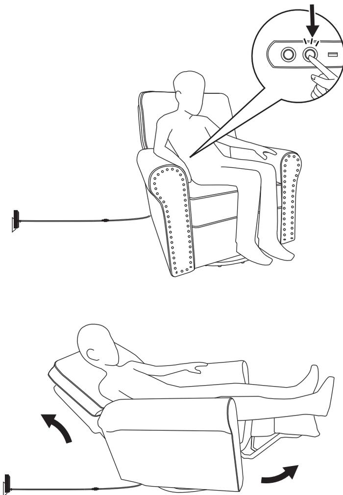
The chair can be made to recline by simply pressing the button located at the inside right of the armrest.
