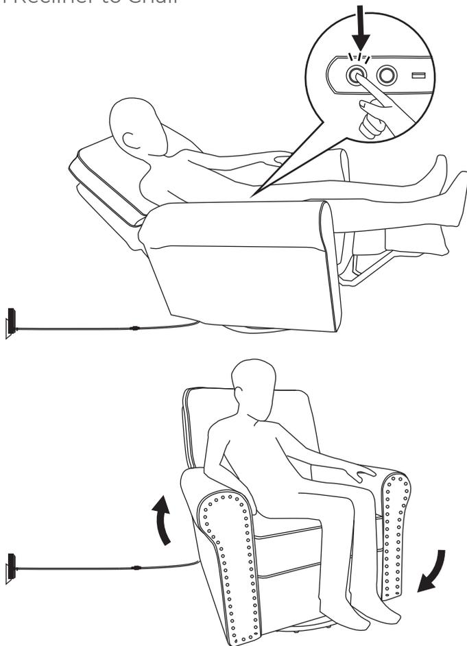
The chair is returned to the upright position by pressing the button located at the inside right of the armrest.
