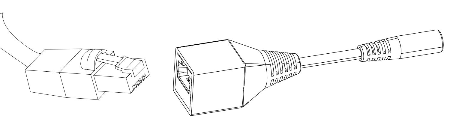
12. Connect the Provided DC Power Adapter into the wall and connect the barrel connector to the other end of of the RJ-45-DC adapter.
