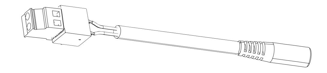
11. Connect the Provided DC Power Adapter into the wall and connect the barrel connector to the other end of the Phoenix adapter.
