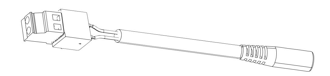
10. Connect the Provided DC Power Adapter into the wall and connect the barrel connector to the other end of the Phoenix adapter.
