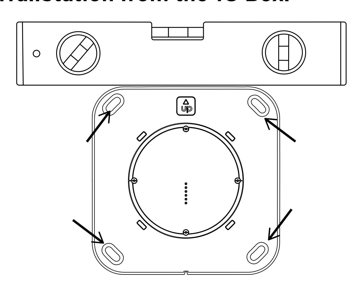
5. Screw the 4 provided anchors into the wall where marked.
