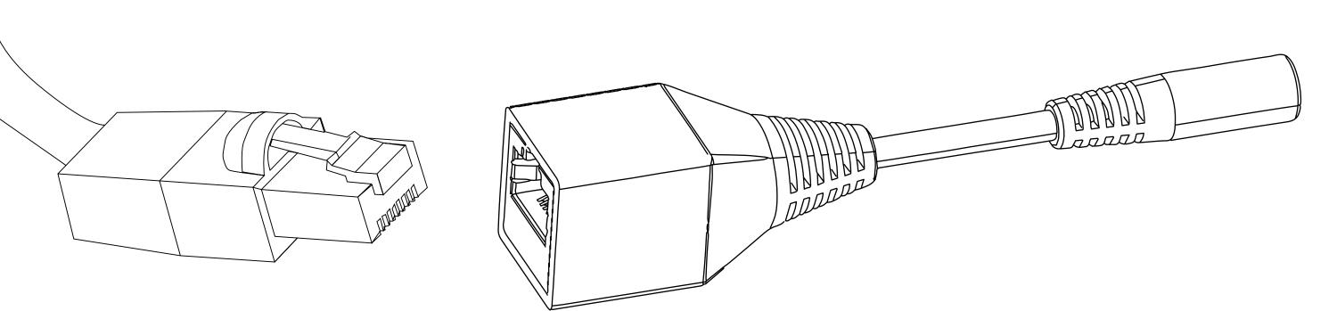
10. Connect the provided DC power adapter into the other end of the RJ-45 DC adapter and plug in the power adapter into an AC outlet.
