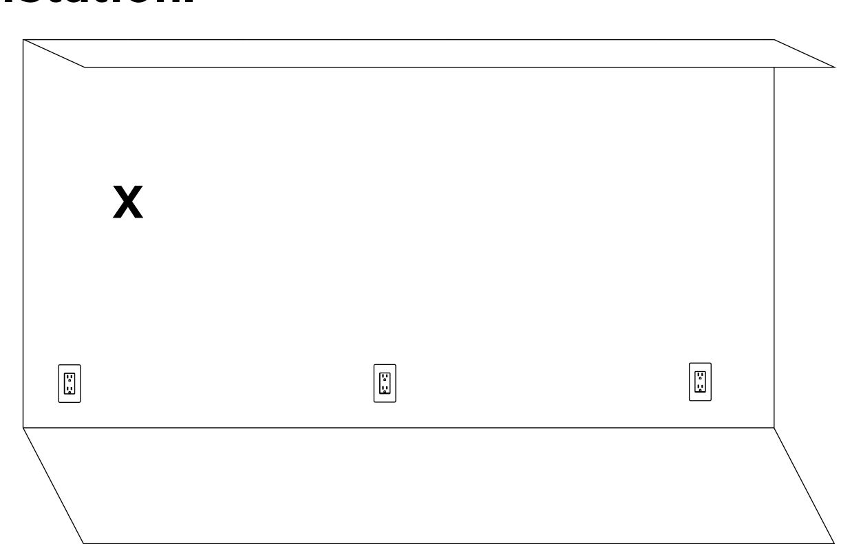
Use a 2-3/4" (70mm) hole saw to cut a hole in the desired location of the WallStation.
