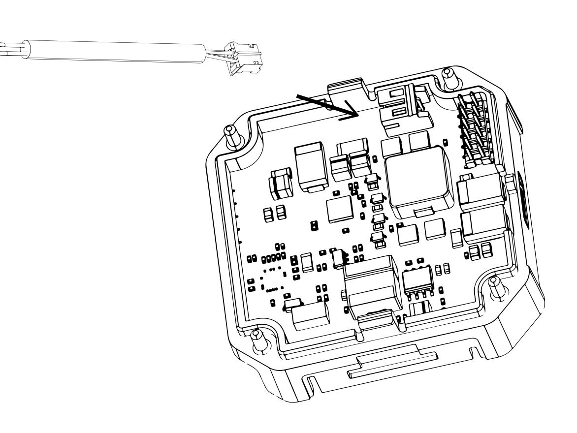
Zip tie the Connector to the DC board for added cable retention.
