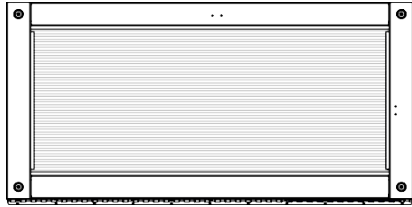
WA01 ENSEMBLE FENÊTRE - W2A04011 (x1) 1 7/8"x19 5/8"x39 3/16" (48x498x996)
