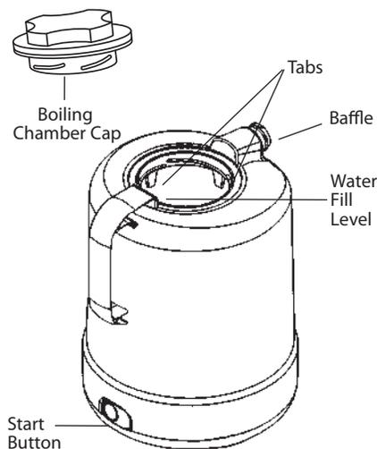
the securing nut, with baffle properly in place, onto the boiling chamber before each use. Failure to properly secure the baffle and nut may result in leakage or early shut off of the distiller.
