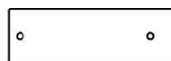
M21 | LISSE MURALE - W4L16057 (x2) 5/8 po x 3 3/8 po x 10 1/2 po (16 x 86 x 268)
