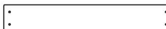
M73 | SUPPORT ARRIÈRE - W4L16070 (x1) 5/8 po x 3 3/8 po x 21 po (16 x 86 x 532)
